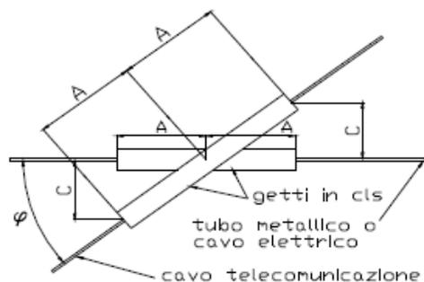
PARALLELISMO FRA CAVO TLC E CAVO ELETTRICO O TUBAZ. METALLICA CON PROTEZ. CATODICA.
